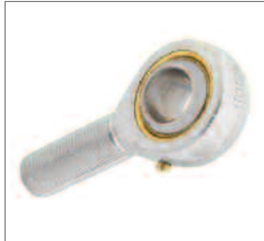
PART NUMBER OEMPB.. NOMINAL RANGE 5mm-30mm COUPLING SURFACES CHROMED STEEL / BRONZE LUBRICATION NOT REQUIRED
