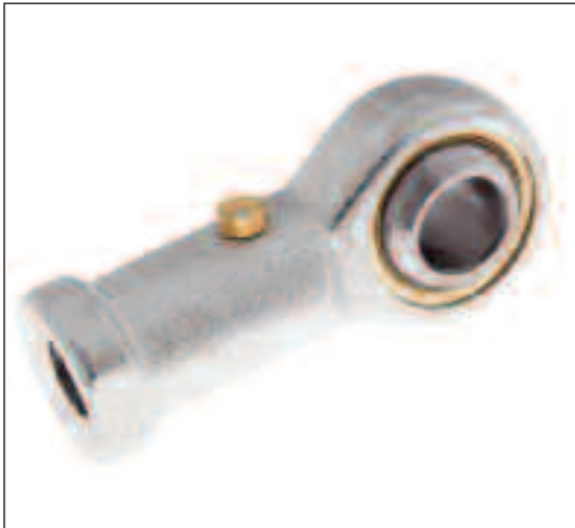
PART NUMBER OEFPB.. NOMINAL RANGE 5mm-30mm COUPLING SURFACES CHROMED STEEL / BRONZE LUBRICATION NOT REQUIRED
