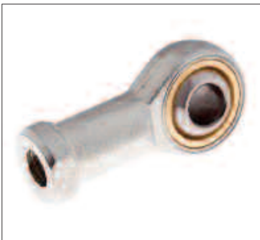
PART NUMBER OEFPW.. NOMINAL RANGE 5mm-30mm COUPLING SURFACES CHROMED STEEL / PTFE LUBRICATION NOT REQUIRED
