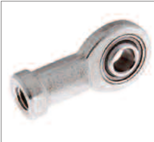
PART NUMBER OEFUK.. NOMINAL RANGE 6mm-80mm COUPLING SURFACES CHROMED STEEL / PTFE LUBRICATION NOT REQUIRED
