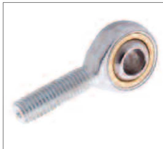
PART NUMBER OEMPW.. NOMINAL RANGE 5mm-30mm COUPLING SURFACES CHROMED STEEL / PTFE LUBRICATION NOT REQUIRED
